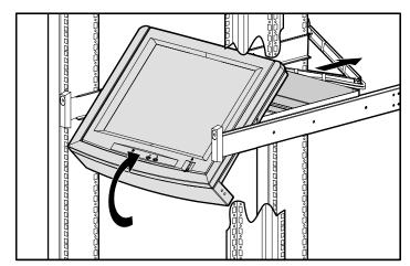
Figure 2-11. Using the retractable tray
